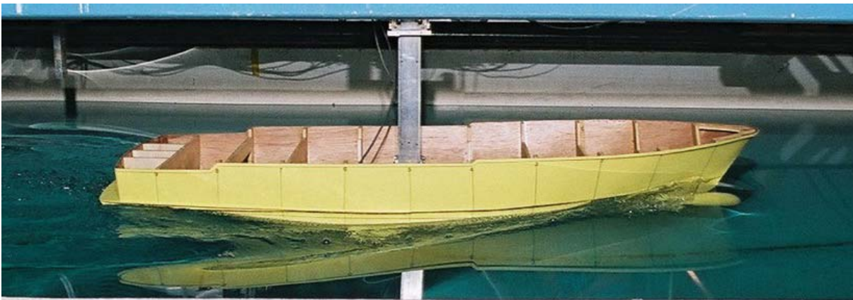
Bray Trawler Hull at 13 knots
