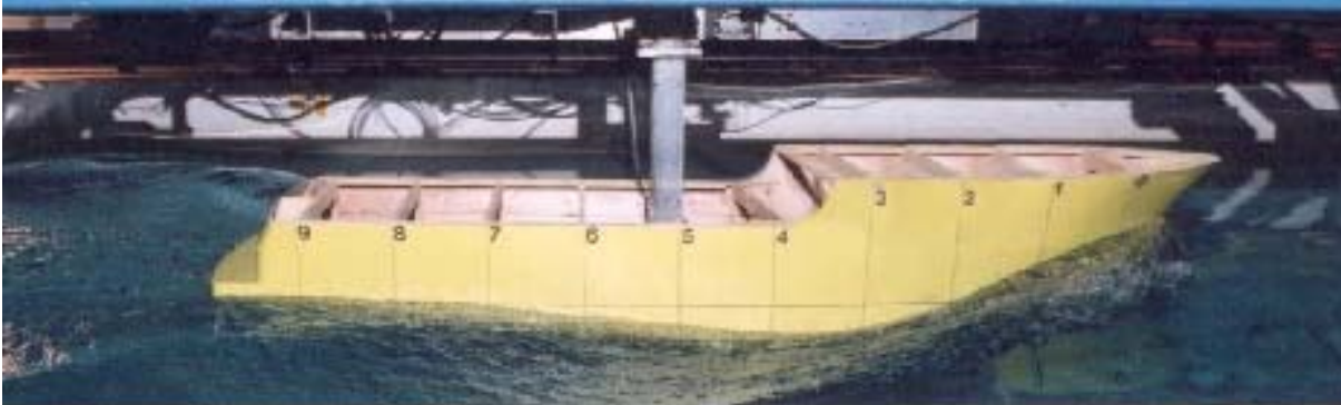
Typical Trawler Hull at 13 knots
