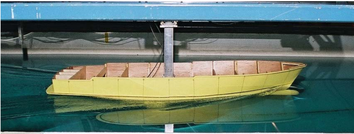
Bray Trawler Hull at 10 knots
